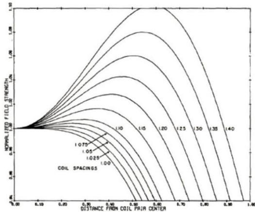
Graph 1. Varying Uniformity of  $B$  with varying distance between the pair of coils.
