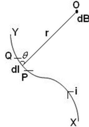
Fig. 1. Magnetic Field near a current carrying conductor
