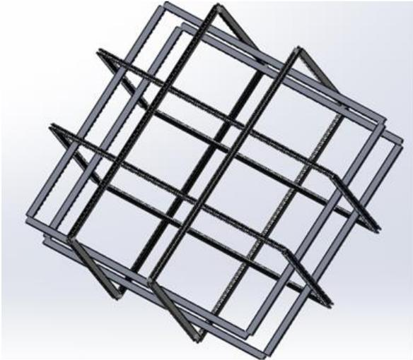
Fig. 4: CAD Model of the proposed Helmholtz Cage
