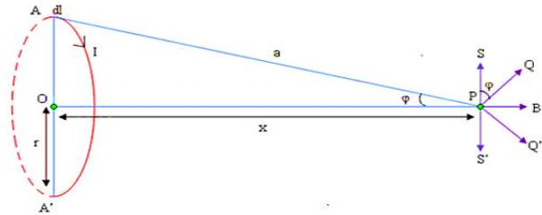
Fig. 2. Magnetic Field at an axial point of a circular coil
